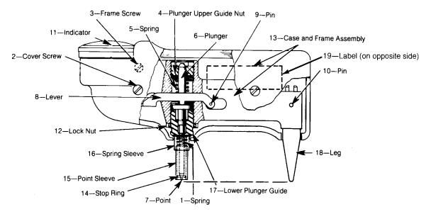
Figure 1. Impressor Cutaway
