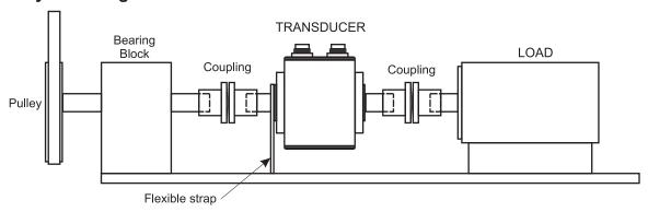
When using a pulley or pulleys it is recommended a bearing block or blocks should be used to ensure bending loads are not transmitted to the transducer. Care should be taken not to induce any end loads or bending moments to the shaft, as these may induce inaccuracies to the torque measurement and in extreme cases damage the transducer.
