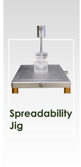
The jig is used to test the Spreadability of butter, margarine, fat, cream lotion, cheese spreads, chocolate spreads and pastes
