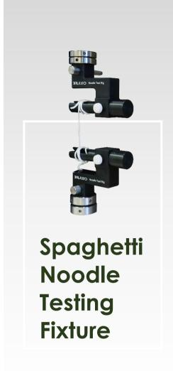
The set consists of two roller grips, designed for tensile testing of food products such as spaghetti and noodles.
