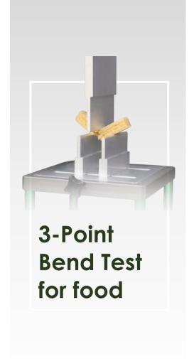
Three point bend jig for general purpose food sample fracture testing.
